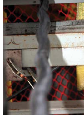
Failing cable due to the “corkscrew” effect
