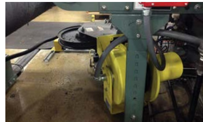
Failing cable due to the “corkscrew” effect
